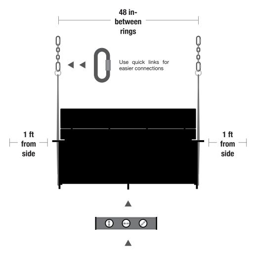
Check that the swing hangs level. Use a level on the swing seat for best measurement.
